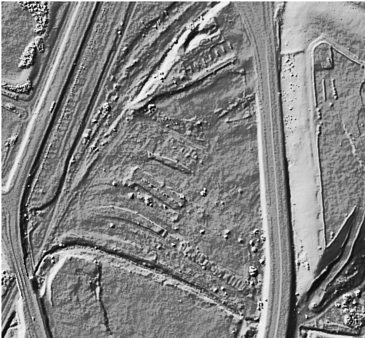
Plate 17A-16: LiDAR Imagery Showing Extent Of Railway Sidings And Structural Foundation Remains Of Redcar Iron Works
